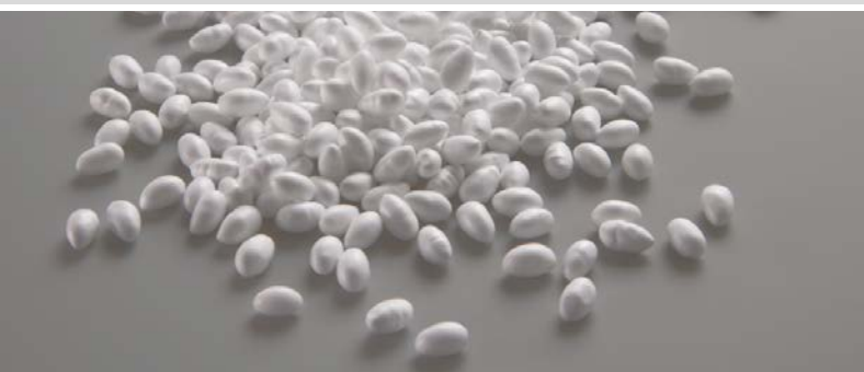
The individual Infinergy® SP beads are sized from 5 to 10 mm and supplied with a bulk density of approximately 110 kg/m 3 .
